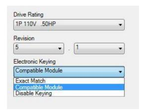
Change response to a configuration problem, i.e. fault the VFD
